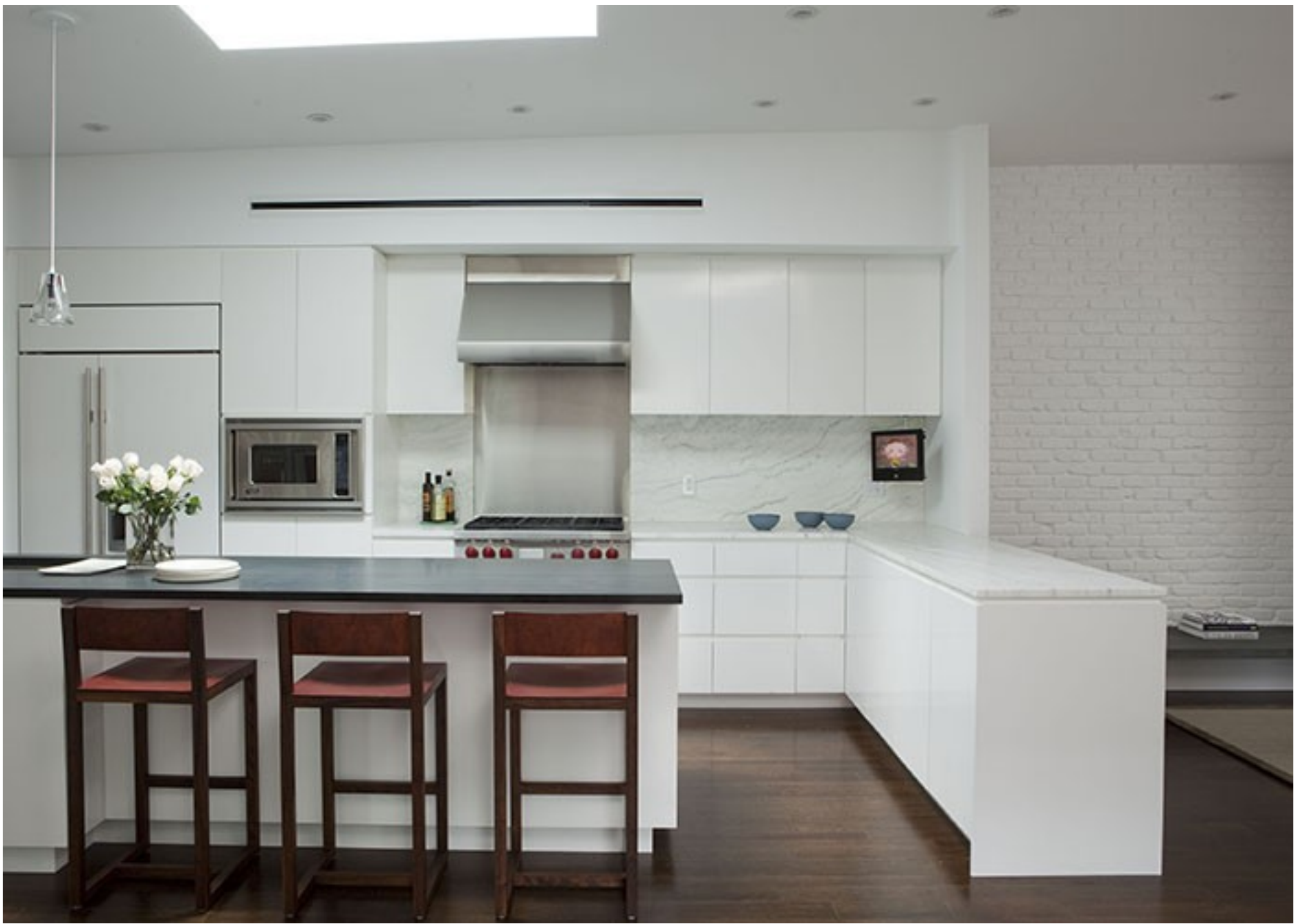
Above: The kitchen cabinets were custom made by New Jersey Hardwoods ( http://www.newjerseyhardwoods.com/home.html ) (introduced to the architects by general contractor Showcase Construction), and are sprayed with an opaque catalyzed lacquer—a hardy finish. The island countertop is honed black Concordia, a type of schist stone ( http://en.wikipedia.org/wiki/Schist ), and the perimeter countertops and backsplash are Olympian Danby marble.
